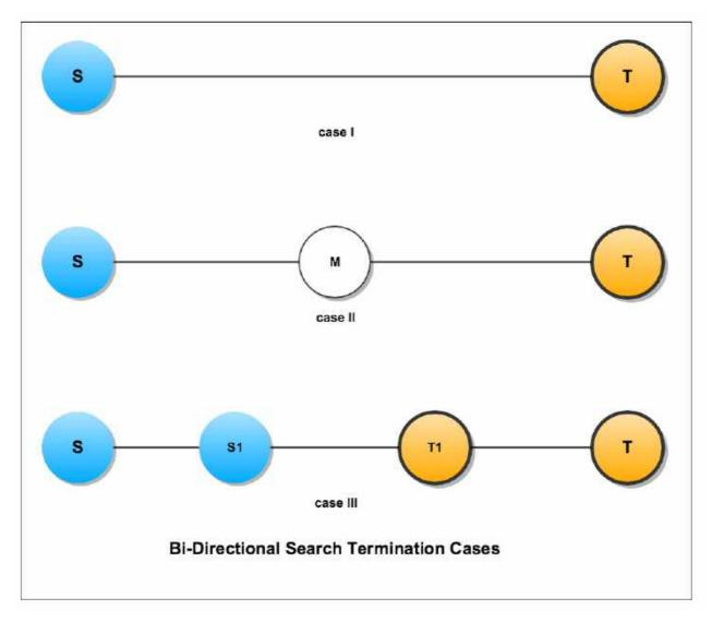
Figure 7 : Three cases for terminating a bi-directional path search.
