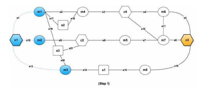
Figure 3: This is the graph after one step. We have traveled from c1 to all of its neighbors, labeling them as visited. For each one that we visit, we update its @pathResult accumulator value in order to keep track of our path as we traverse the graph.
